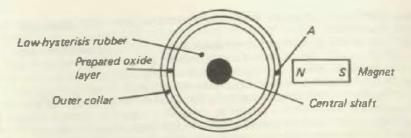
'direction' field in accord with the direction of rotation. For the arrangement shown above, clockwise rotation will ensure ascent.
